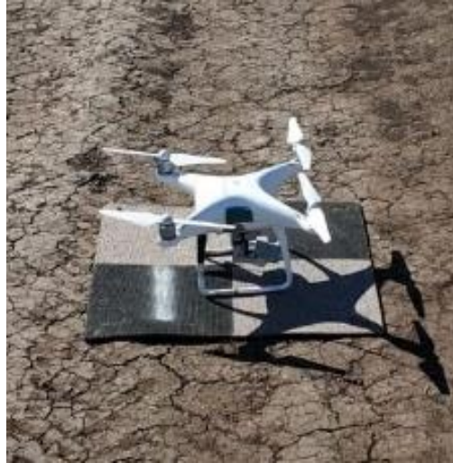
Plate 3-2 Phantom 4 Advanced with an RGB camera sitting on a GCP mat.
