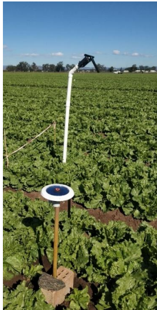
Plate 3-1 Setting up the two devices in the paddock (top: time-lapse camera; bottom: Arable Mark 2 sensor).
